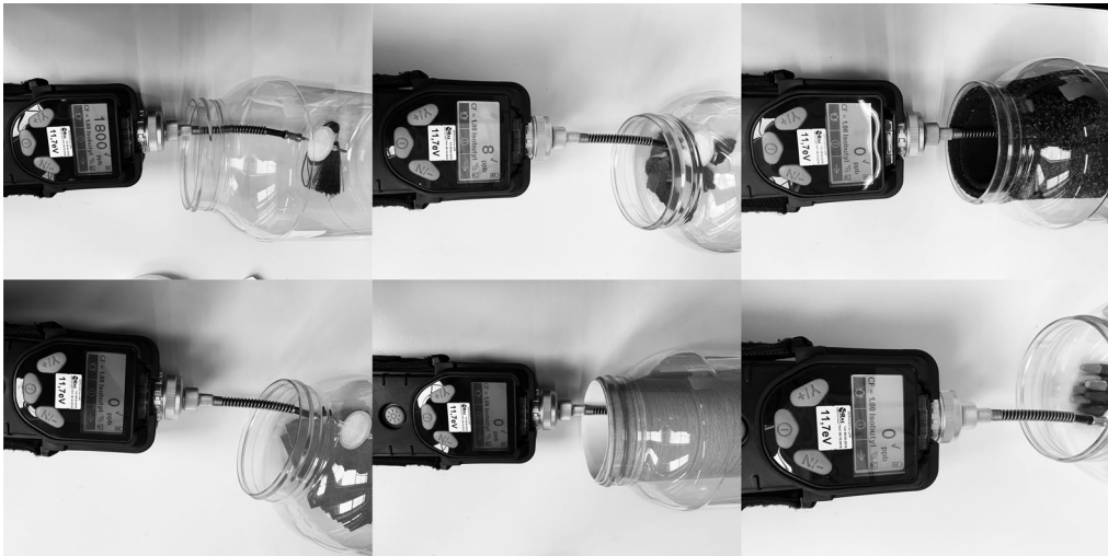
Figure 5. VOCs emitted by the selected materials: (a) perfume; (b) mint leaves; (c) carpet; (d) MDF; (e) vinyl; and (f) crayons.
