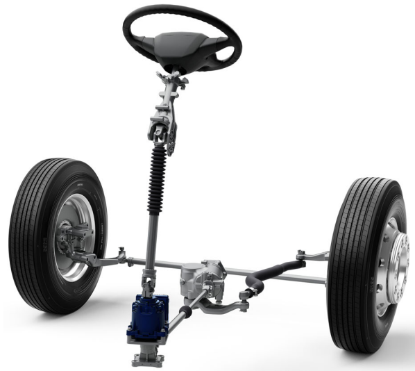
Figure 1. Schematic illustration of VDS. Note: VDS = Volvo dynamic steering
