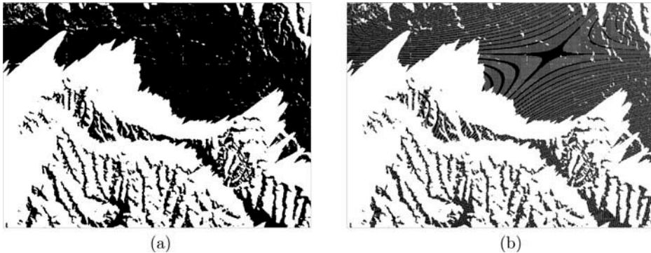
Figure 14. Optimized float implementation (a) versus naive float implementation (b) of the loop in the kernel.
