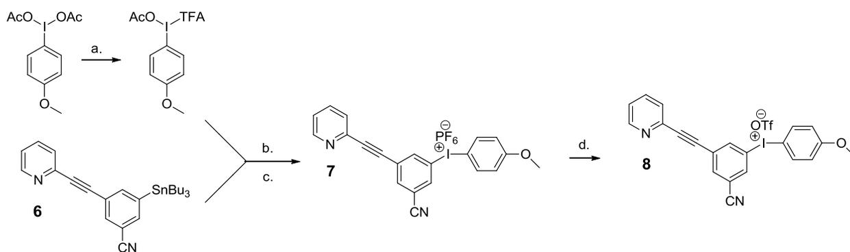
**Scheme 8.** Iodonium chemistry of PEB. Reagents and conditions: (a) TMS-TFA acetonitrile; (b) CH<sub>3</sub>CN, 40 °C, 14 hrs. (c) H<sub>2</sub>O, NaPF<sub>6</sub>; (d) Ion-exchange column.
