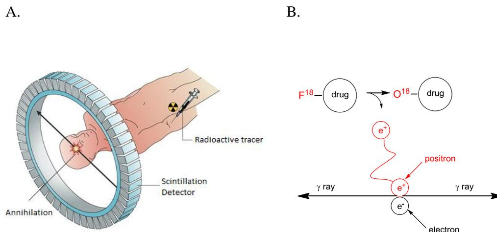
**Figure 2.** PET imaging. A. Schematic diagram showing the process and apparatus for collecting a pet scan. Modified from Nature Reviews, 4, **June 2004**, 457-469. B. Cartoon showing the nuclear processes leading to the production of gamma rays.
