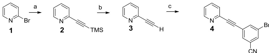
**Scheme 5.** The preparation of 3-bromo-5-((6-methylpyridin-2-yl)ethynyl)benzonitrile
