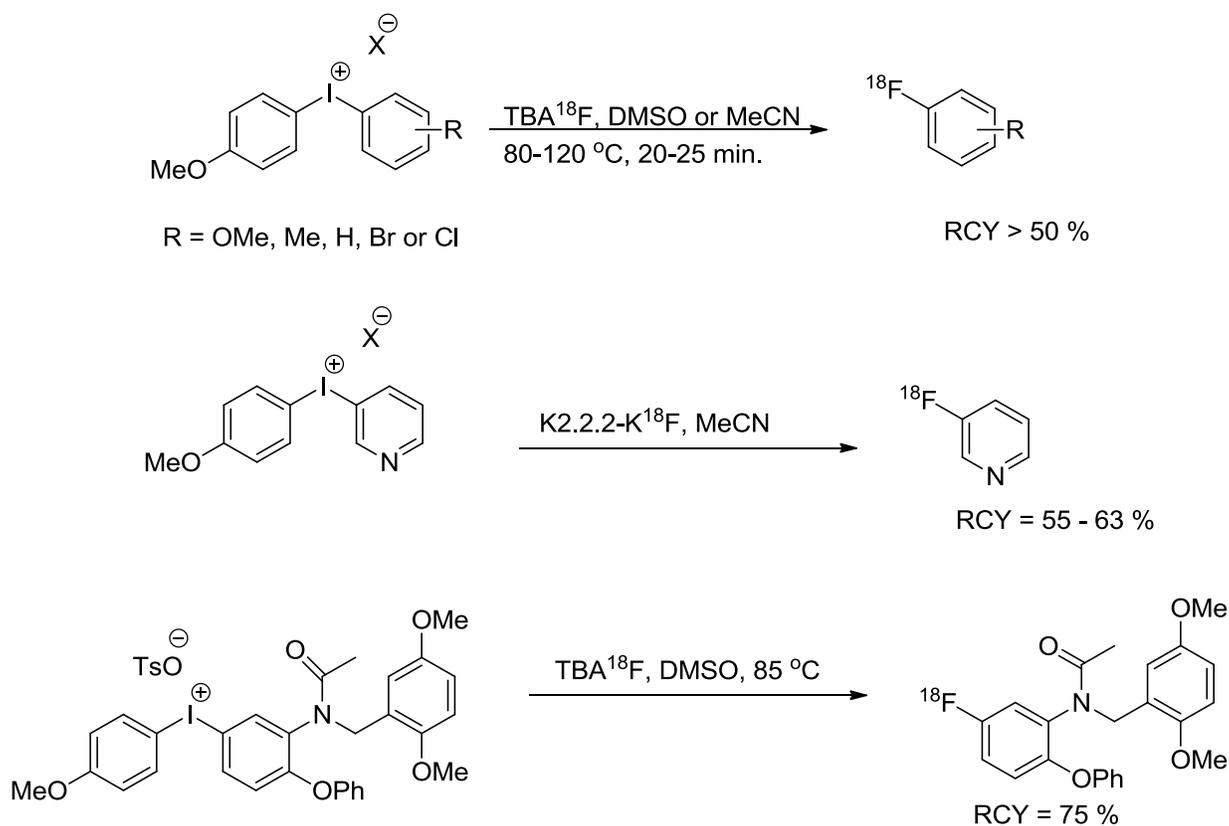
**Scheme 3.** Some examples of radiofluorination with Diaryliodonium salts.<sup>1</sup> RCY is decay-corrected radiochemical yield.
