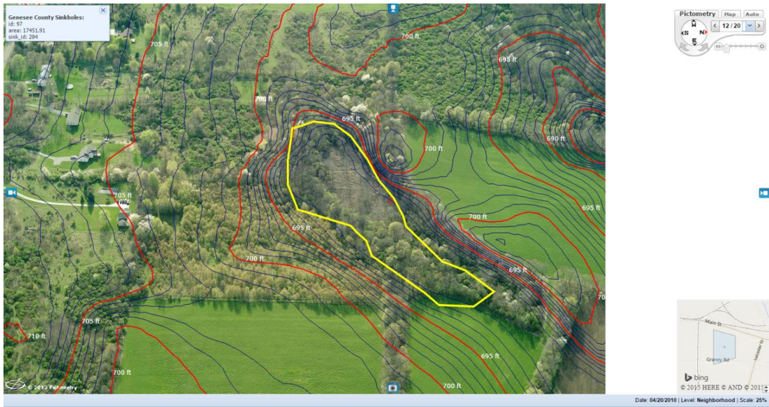
Figure 4a. This is dry-period time-step of Sinkhole #97 in Caledonia, NY. This feature is a very evident sinkhole feature, lying nicely within the contours. It appears to be a dry pond basin, possibly a vernal pool that refills with snowmelt. View from the east.
