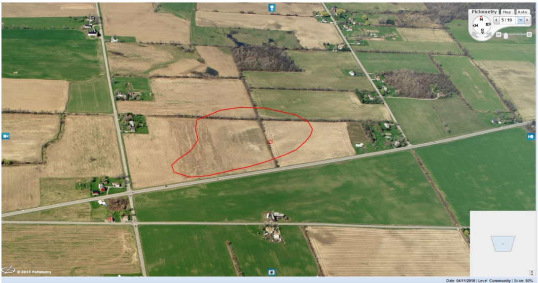
Figure 15b. Dry time-step of Sinkhole #25. Although absent of water, the Ivison Rd. disappearing lake still shows signs of soil discoloration, likely due to enhanced sub-surface moisture.
