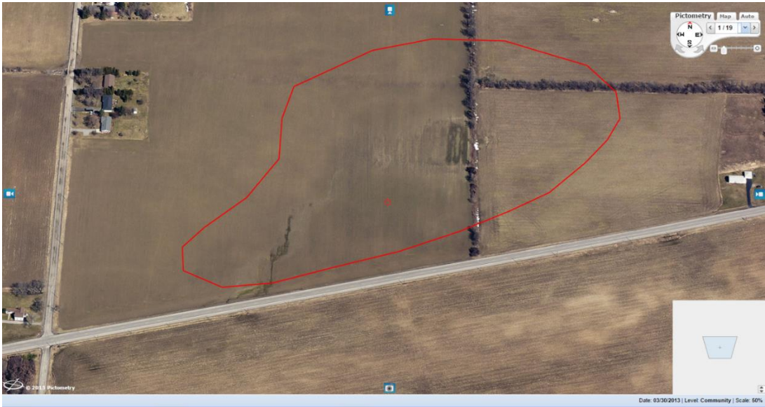
Figure 15a. Moist time-step of the disappearing lake at Ivison Rd. in Sinkhole # 25. Not only is there ponding at the very center, but visible ‘stream’ formation is seen in the southwest portion of the feature.
