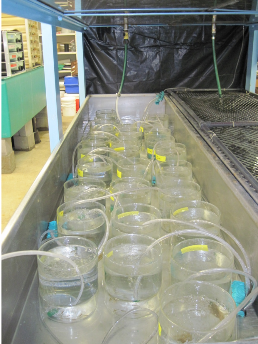
Figure 5. Aquaria used to determine alevin survival from hatching to swim-up stage. Each aquarium contains alevins from one specific female fish.
