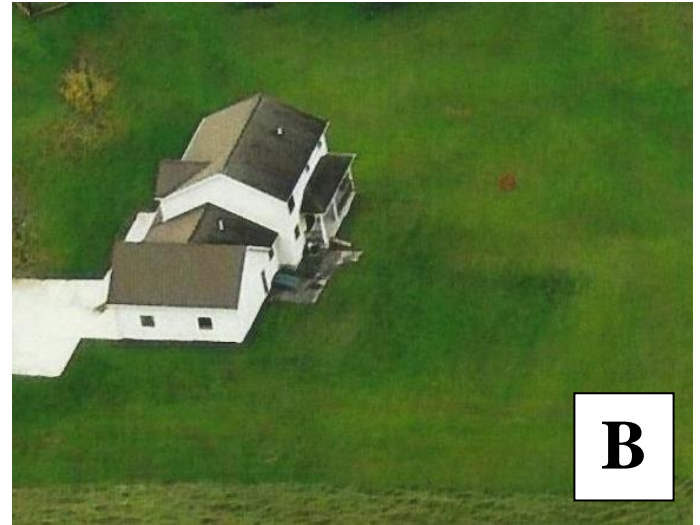
Figures 1A, 1B, and 1C. Images A and B show the darkening of grass where the septic field is. Image C shows the gathering of leaves over the septic field due to micro-relief.
