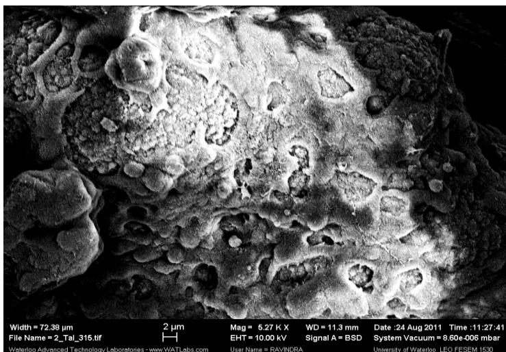
Figure 4.25: SEM images for homo-polymer produced with TEAL and ES-70 silica
