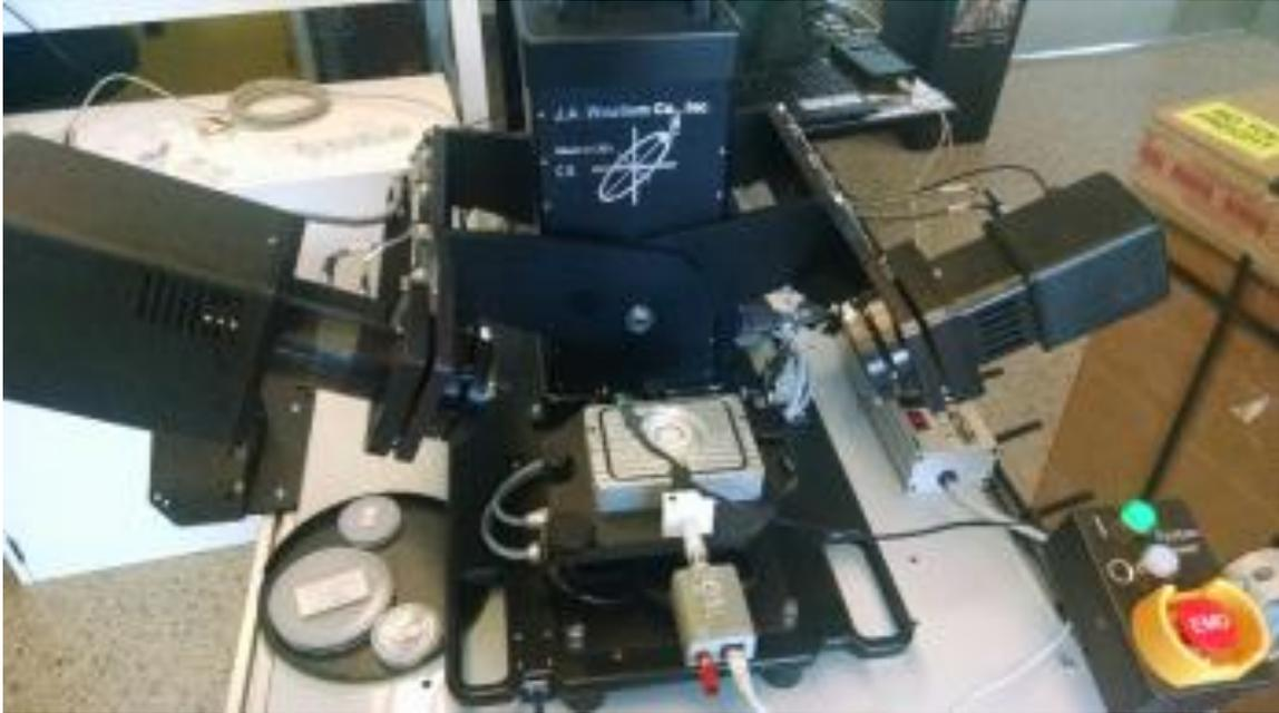
**Figure 7.1: Combined QCM (water uptake) and ellipsometry (thickness) setup.**
