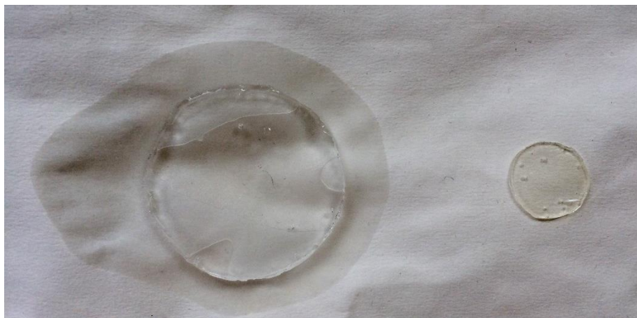
Figure 11: 2:8 SHMeMB:AM hydrogel with 1.5 mol% crosslinker after swelling (left) and before, i.e. as prepared (right).
