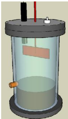
Figure 10. Sediment Oxygen Demand Reactor Design
