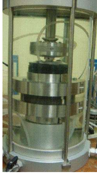
Figure 4.5: Complete set up of new integrated porous rigid wall and flexible wall permeameter.
