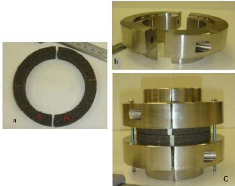
Figure 4.6: Components of newly designed permeameter (1a) Porous stone cylinder (2a) Stainless steel porous stone holding cap (2c) porous stone with clamped holding cap.
