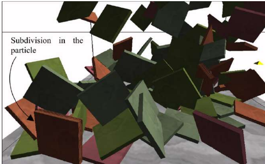
Figure 3.22: Discrete Element Model (DEM) showing evolution of microstructure in montmorillonite, particles decrease in size with increasing swelling (Katti et. al., 2009).
