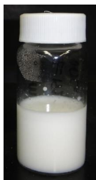
FIGURE 4.1 – IIR-VImBr emulsion following sonication and the removal of organic solvents
