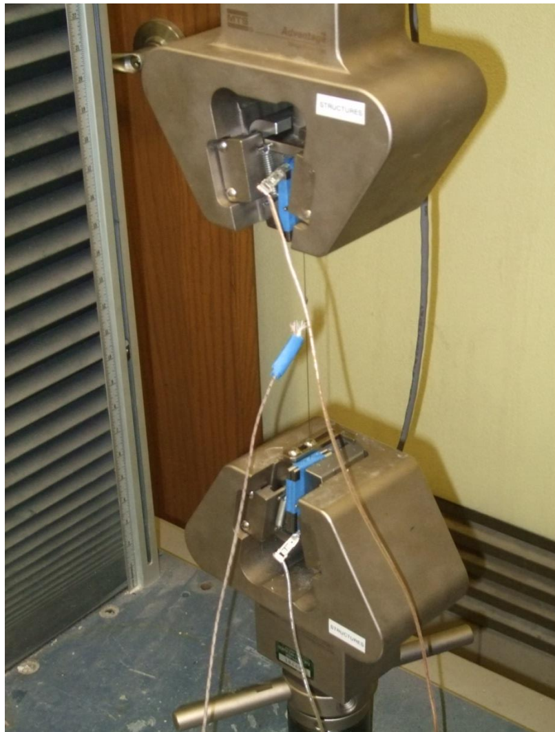
Figure 4.2: Test Set-up of SMA Wire Specimen
