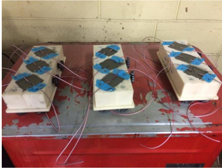
Figure 10. The 2 inch cubic mold for sample fabrication
