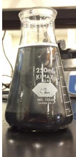
Figure 4. CNTs in water using direct mixing method
