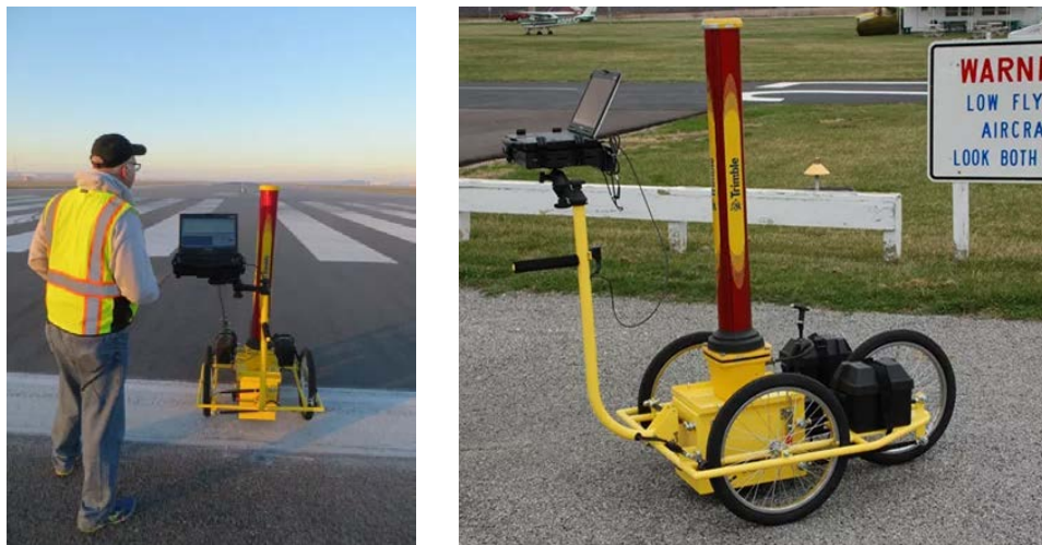
Figure 3. Rod and level pavement profiler (Consultants, 2018)
