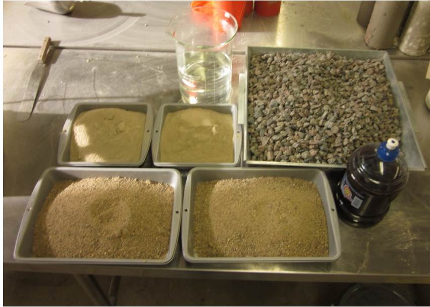
Figure 3.16. Preparing the Mixture Proportion for Concrete Mix
