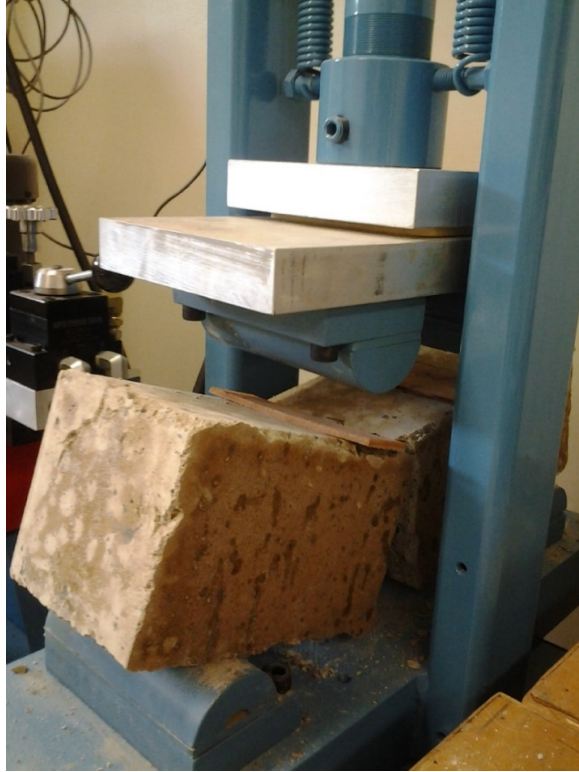
Figure 4.32. Flexural Strength Test of Beam
