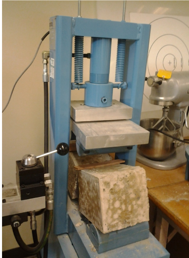
Figure 4.31. Flexural Strength Test of Beam
