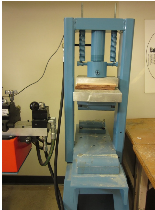
Figure 3.35. Flexural Strength Test Machine of Beam
