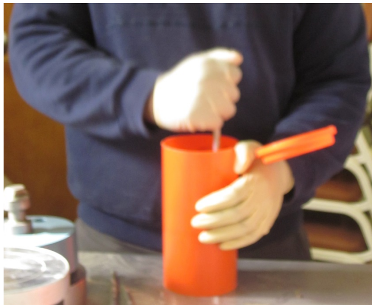
Figure 3.21. Consolidating Concrete using Rod
