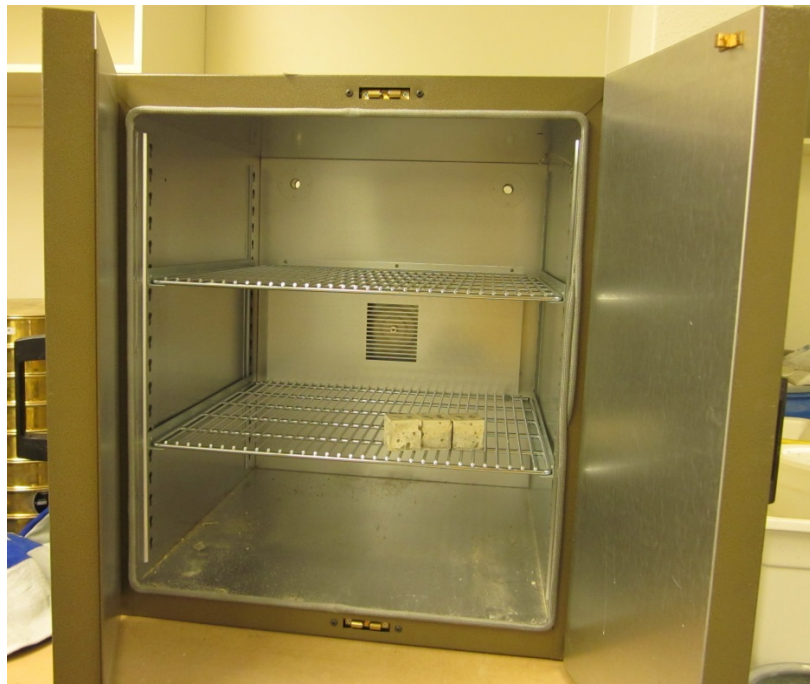
Figure 3.8. Oven for Curing
