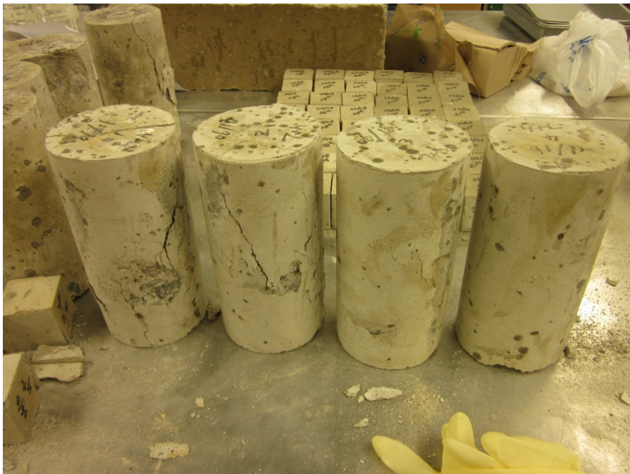
Figure 4.14. Cracks formed after Compressive Strength Test of Cylinders
