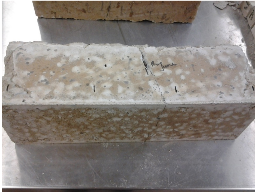
Figure 4.34. Cracks Formed after Flexural Strength Test of Beam
