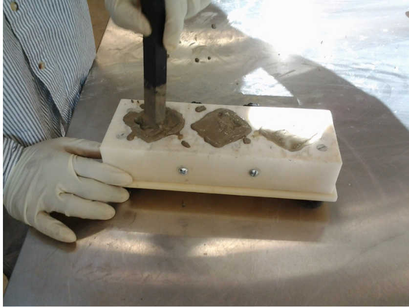
Figure 3.26. Tamping Fresh Mortar in Cube Molds
