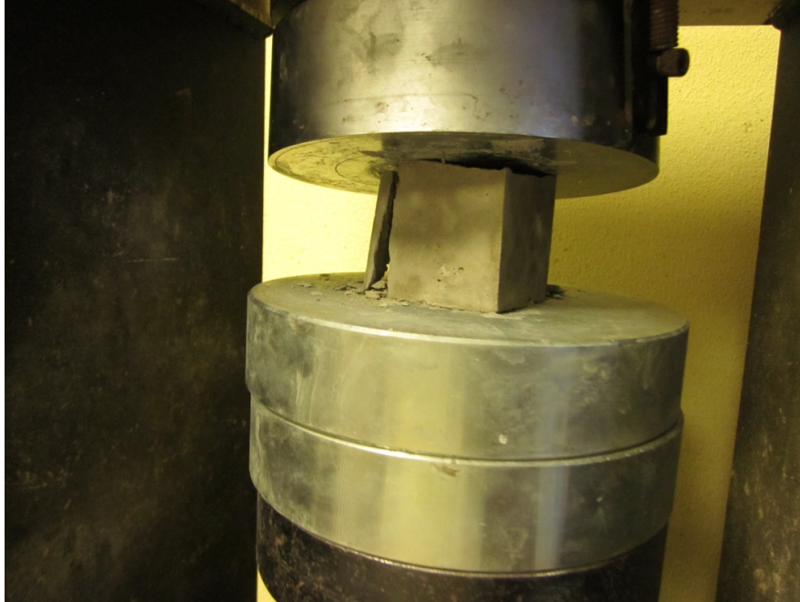
Figure 4.9. Compressive Strength Test for Cube
