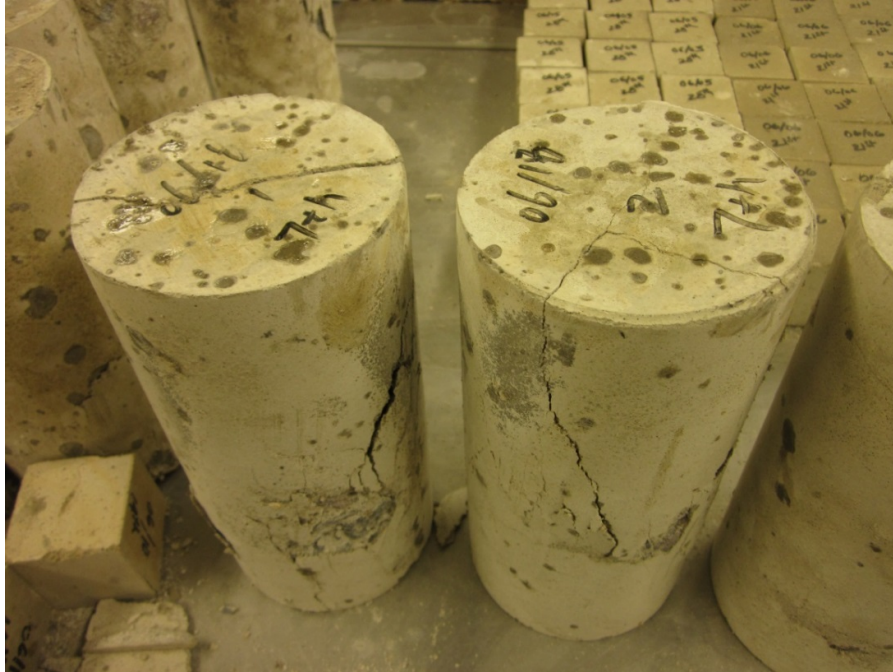
Figure 4.13. Cracks formed after Compressive Strength Test of Cylinders
