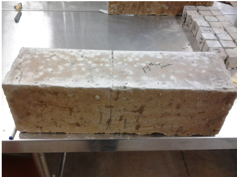
Figure 4.33. Cracks Formed after Flexural Strength Test of Beam
