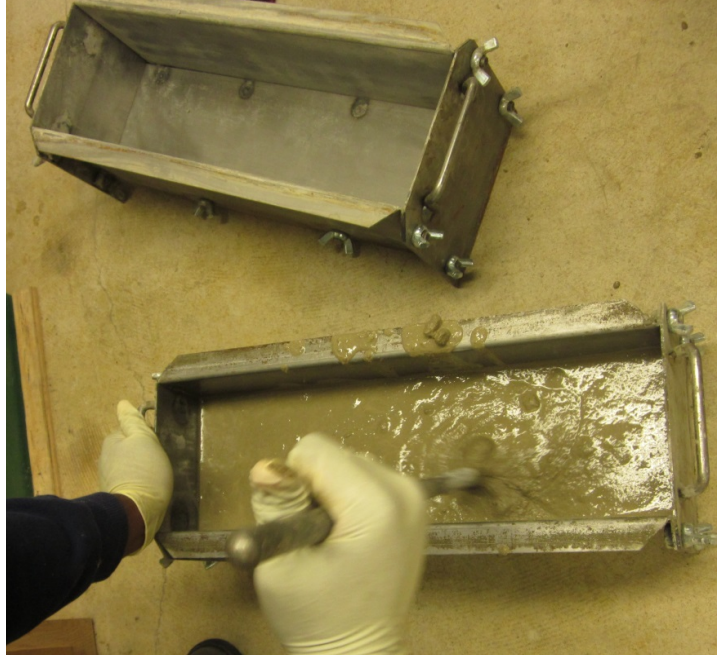
Figure 3.22. Consolidating Concrete using Rod
