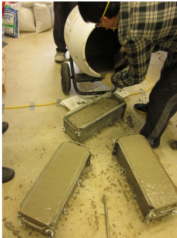
Figure 3.23. Pouring and Leveling Concrete in Beam Mold
