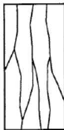
Type 3 Columnar vertical cracking through both ends, no well- formed cones
