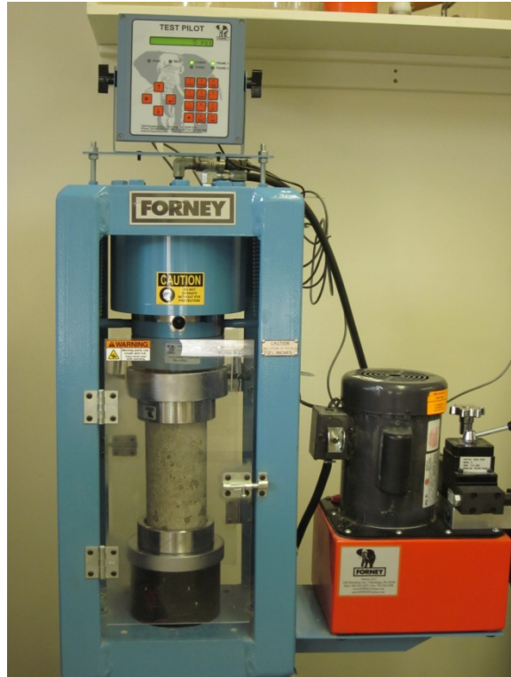
Figure 3.34. Compressive Strength Test Machine of Cylinder Specimen
