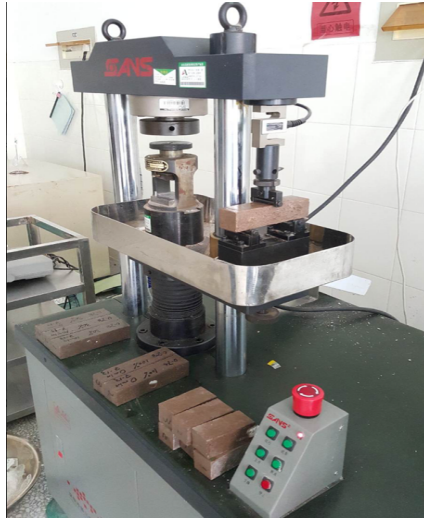
Figure 3.9. The test of flexural strength
