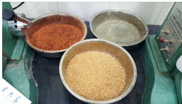
Figure 3.1. Prepared clay brick aggregate, cement and natural fine aggregate (sand)
