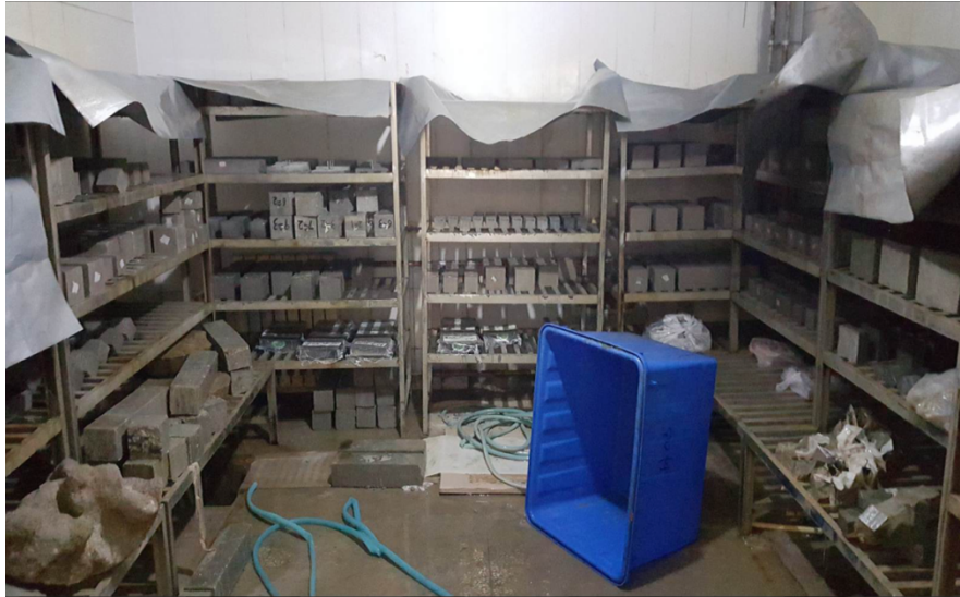
Figure 3.5. The curing room of concrete specimens
