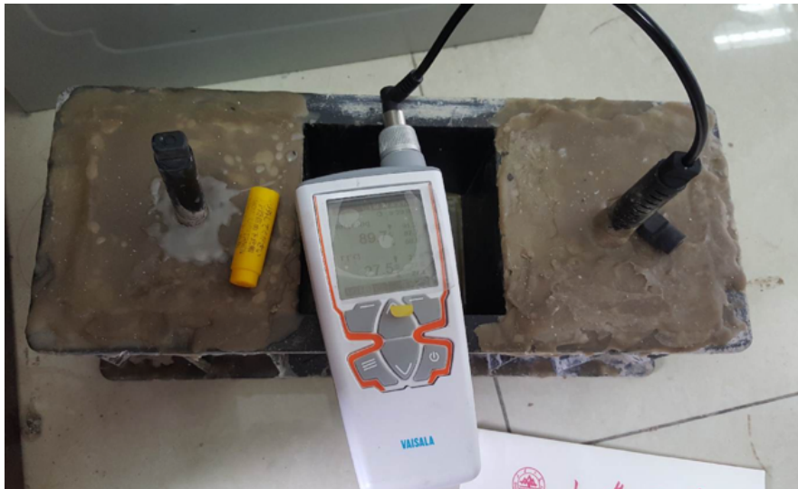
Figure 3.11. The temperature and humidity sensor
