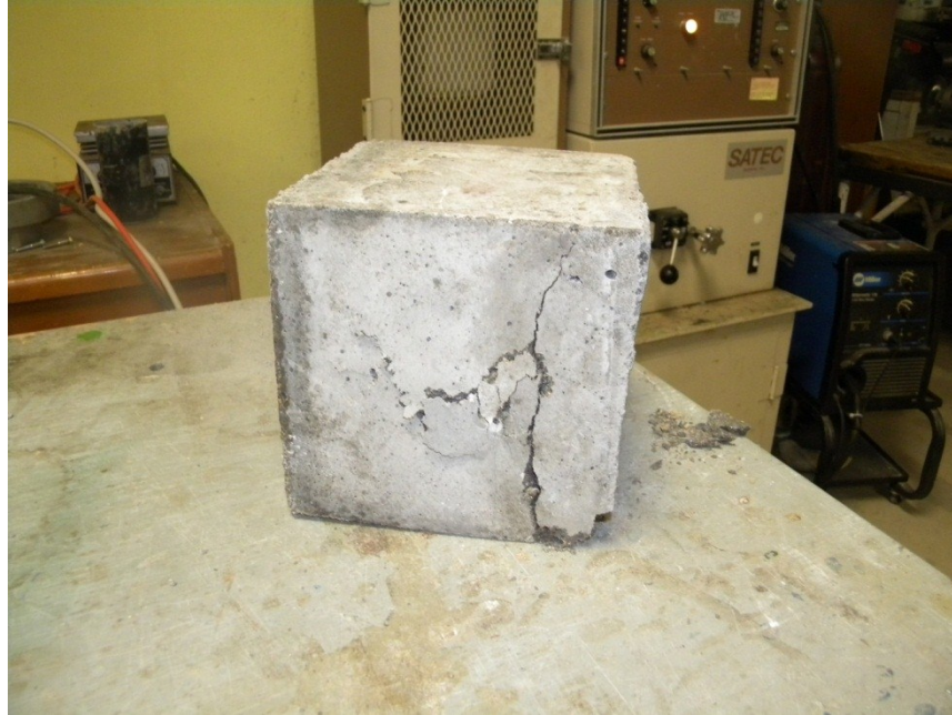
Figure 4.12. The Failure of the cube
