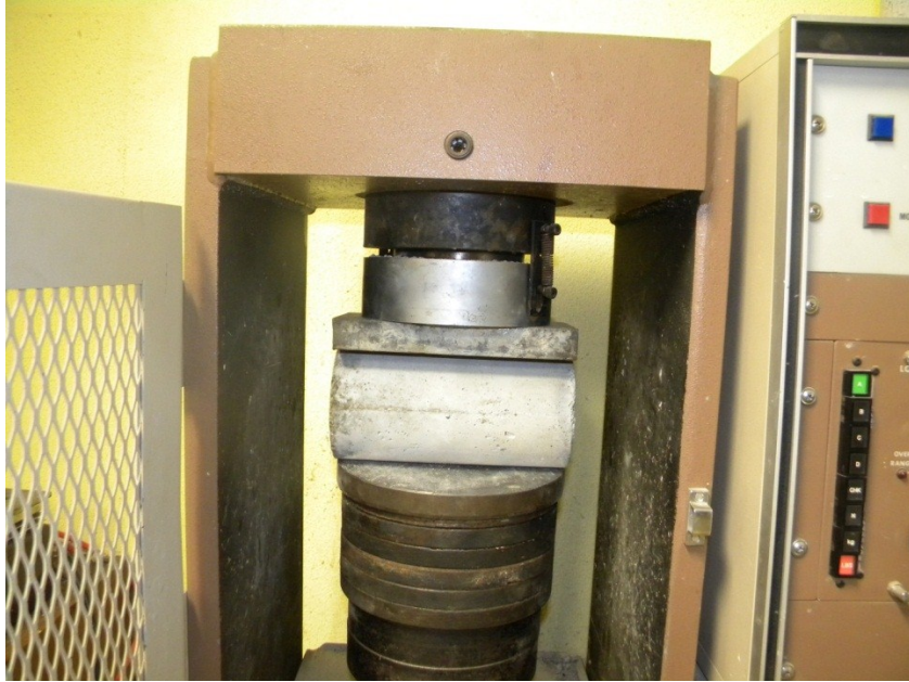
Figure 4.21. Splitting tensile strength for cylinder
