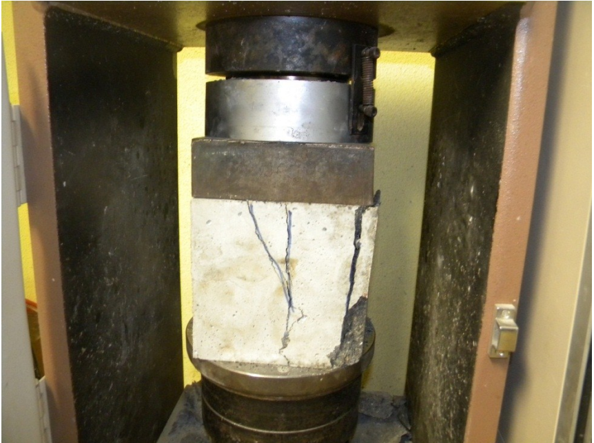
Figure 4.11. The failure of the cube
