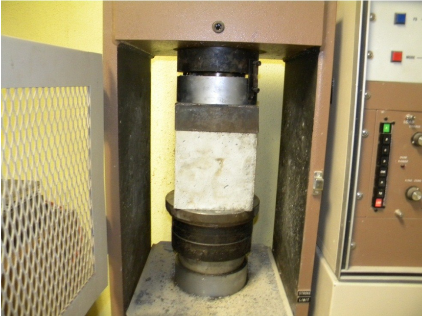
Figure 4.10. The compression test for the cube specimens
