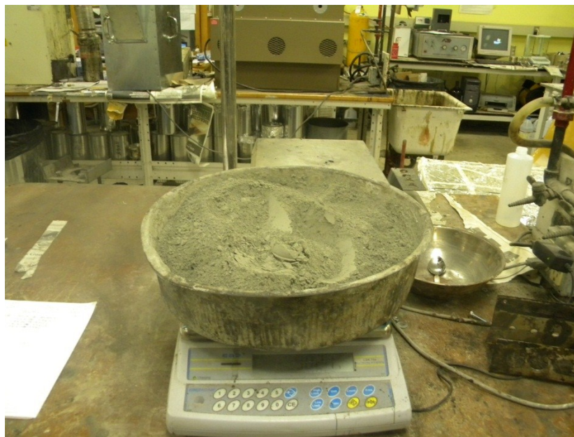
Figure 3.1. Preparing the weight of materials (cement)
