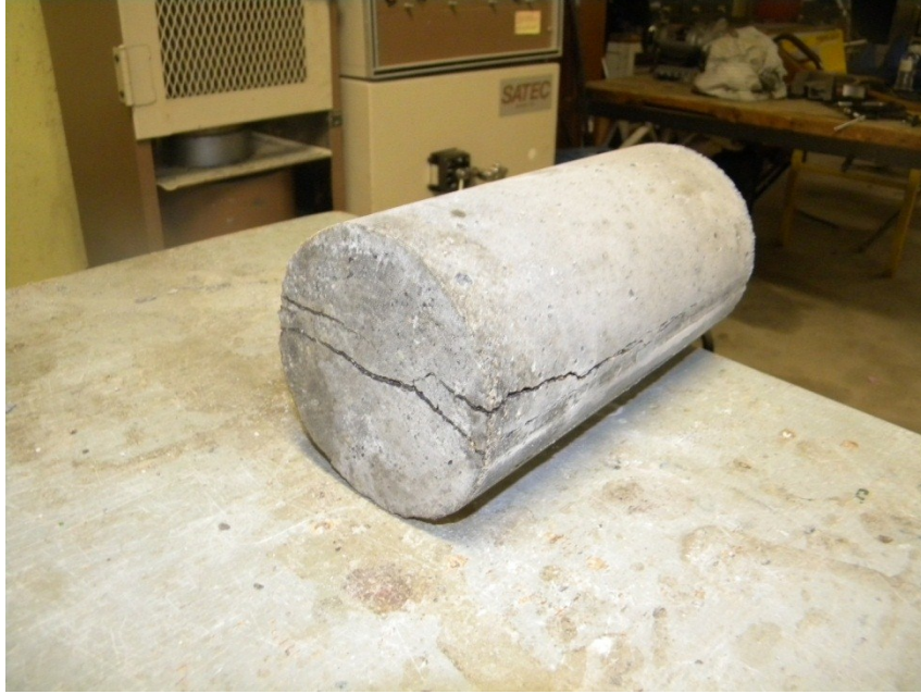
Figure 4.23. The failure (splitting) shape
