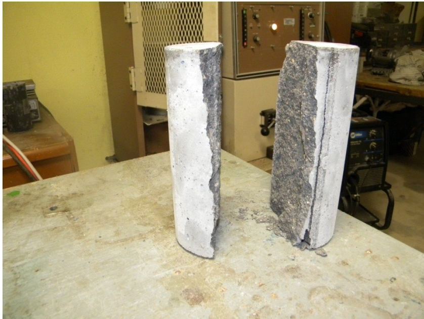
Figure 4.22. The failure (splitting) shape
