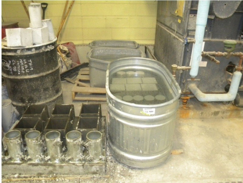
Figure 3.10. The oiled molds with curing tanks
