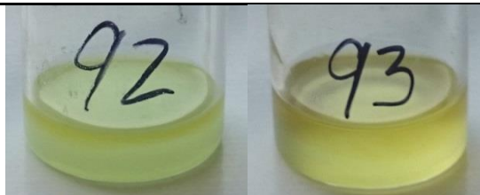
Figure 3-24. Polymerization mixtures of MA [50]:[1]:[0.2] in PPG, 33%v/v (92) and 50%v/v (93), at 30°C
