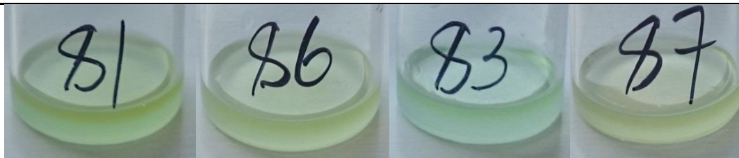
Figure 3-16. Polymerization mixtures of MA in PEG-Ethanol 33% v/v (81, 86) and 50% v/v (83, 87)
