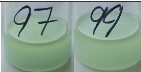
Figure 3-31. Polymerization mixtures of 4K (97) and 10K (99) PMA in 33%v/v 75-25PPG-Ethanol
