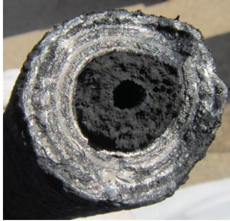
Figure 1 – Radiant coil with significant coke formation
