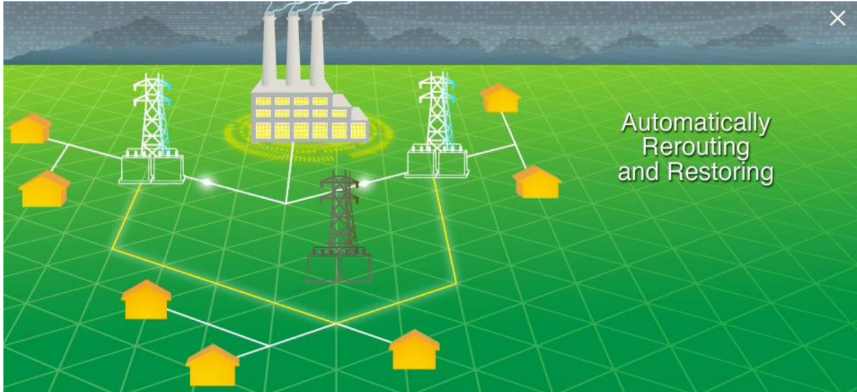
Figure 2.2: Dynamic Electrical Power Rerouting. [2]
