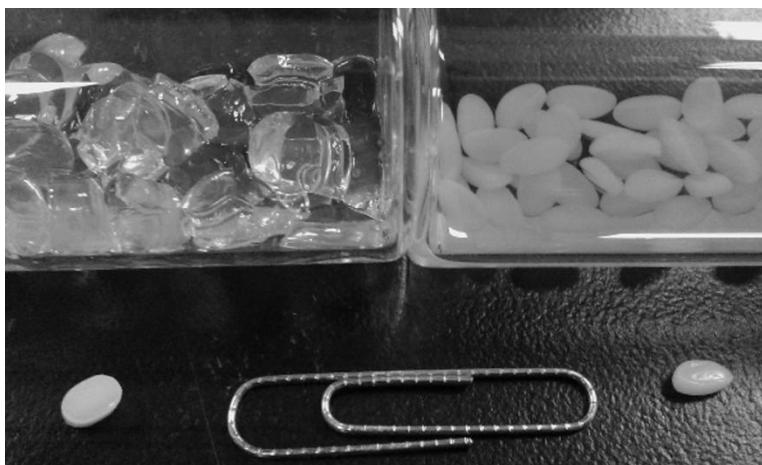
Figure 3-2: Photograph comparing swelling behavior in different grades of Hytrel® when exposed to indene: 3548 swelling and cracking on left, 8206 unaffected on right. Unexposed beads in foreground for comparison with paper clip for scale.
