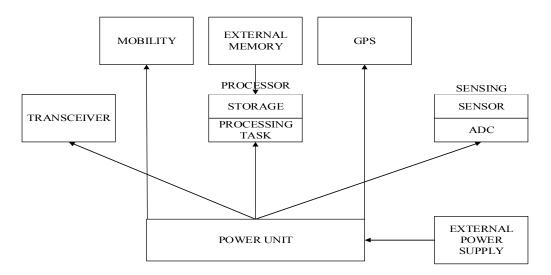
Figure 3-1. Components of a sensor node
