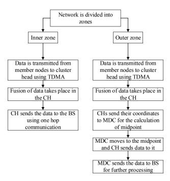
Figure 4-3. Data transmission from sensor nodes to base station [1]
