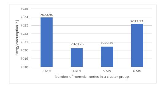
Figure 5-20. Energy consumption of different member nodes in a cluster group
