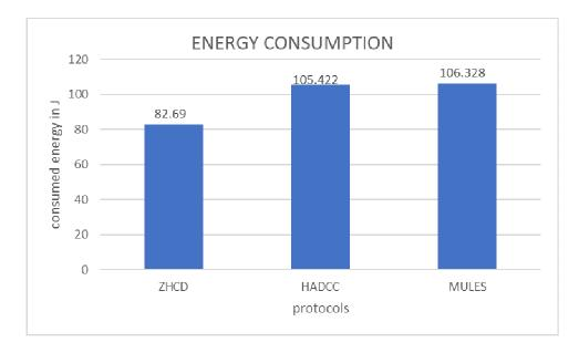
Figure 5-5. Energy consumption of protocols in 25 seconds
