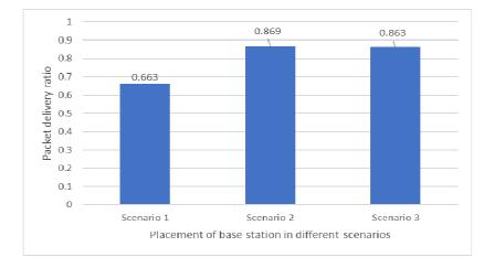
Figure 5-16. Packet delivery ratio of three scenario
