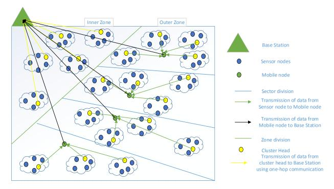
Figure 5-12. Positioning of base station in the corner of network
