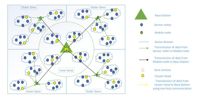
Figure 5-11. Positioning of base station in the center of network
