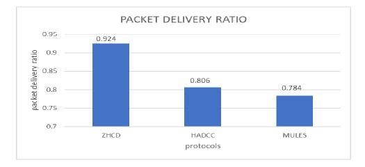
Figure 5-7. PDR of protocols in 25 seconds
