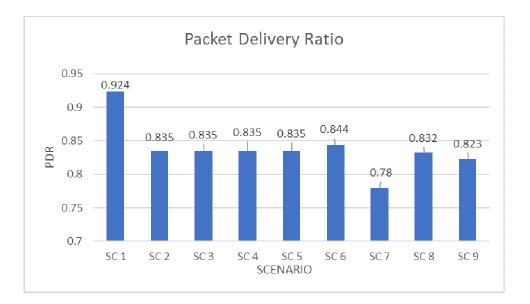
Figure 5-4. Packet delivery ratio of different scenarios
