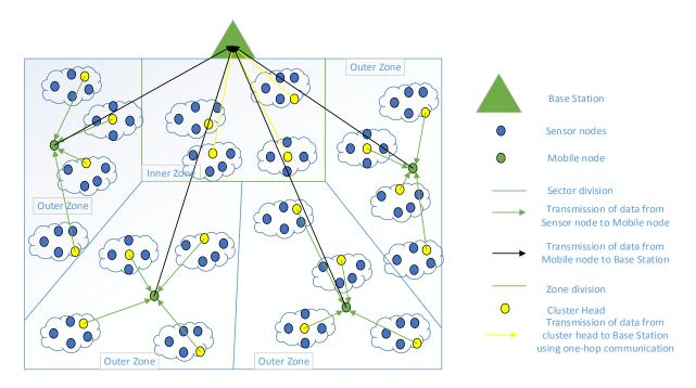
Figure 5-13. Positioning of base station where nodes are dense in the network
