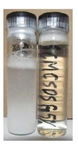
**Figure 3.8:** Photograph showing vials containing 51 mM SDS with 0 wt% (left) and 5 wt% (right) gelatin, refrigerated at 4 °C for 10 days. Adding 5 wt% gelatin appears to have stopped or postponed SDS precipitation for more than 10 days, maintaining gel transparency.
