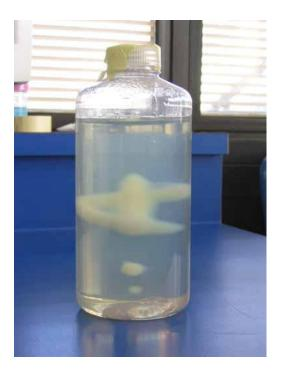
**Figure 2.2:** Photograph of a non-uniformly irradiated polymer gel dosimeter (Koeva 2008), used with permission. The white opaque regions received a higher radiation dose than the surrounding transparent regions in the gel. This dosimeter was irradiated using external Co-60 radiation beams from different directions.
