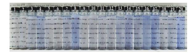
**Figure 4.5:** Photograph of un-irradiated vials (23×85 mm clear glass) containing LCV-CTAB-TCE gels manufactured at varying concentrations of CTAB, LCV, and TCE as described in table 4.11. Vial numbers correspond to the sample numbers in table 4.11.
