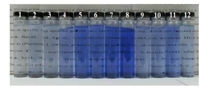
**Figure 4.3:** photograph of un-irradiated vials (23×85 mm clear glass) of gels manufactured using different concentrations of Tx100, LCV, and TCE. Vial numbers correspond to the gel numbers in table 4.9.
