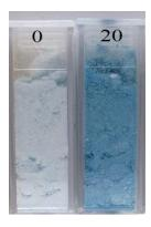
**Figure 3.5:** Un-irradiated PCDA powder and PCDA powder irradiated to 20 Gy.
