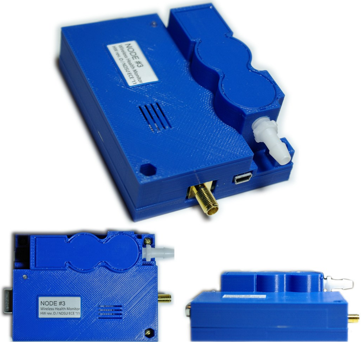
Figure 49. Completely assembled Node device (without external sensors and antenna).
