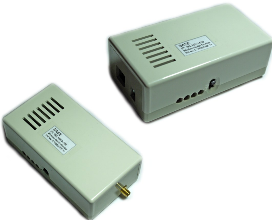
Figure 76. Completely assembled Base device (without power supply, Ethernet connections and attached antenna).
