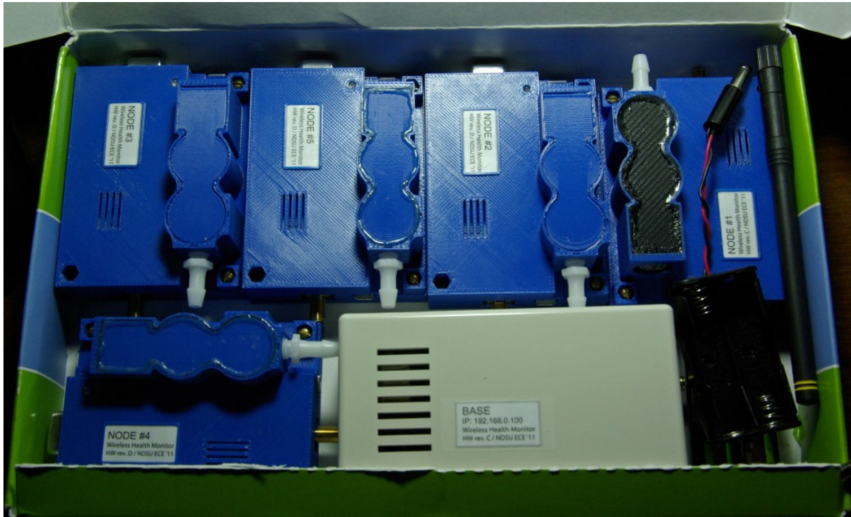
Figure 80. Completely assembled Base and Node devices.
