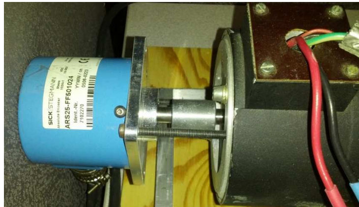
Figure 36. The mechanical connection between the encoder and DC motor.
