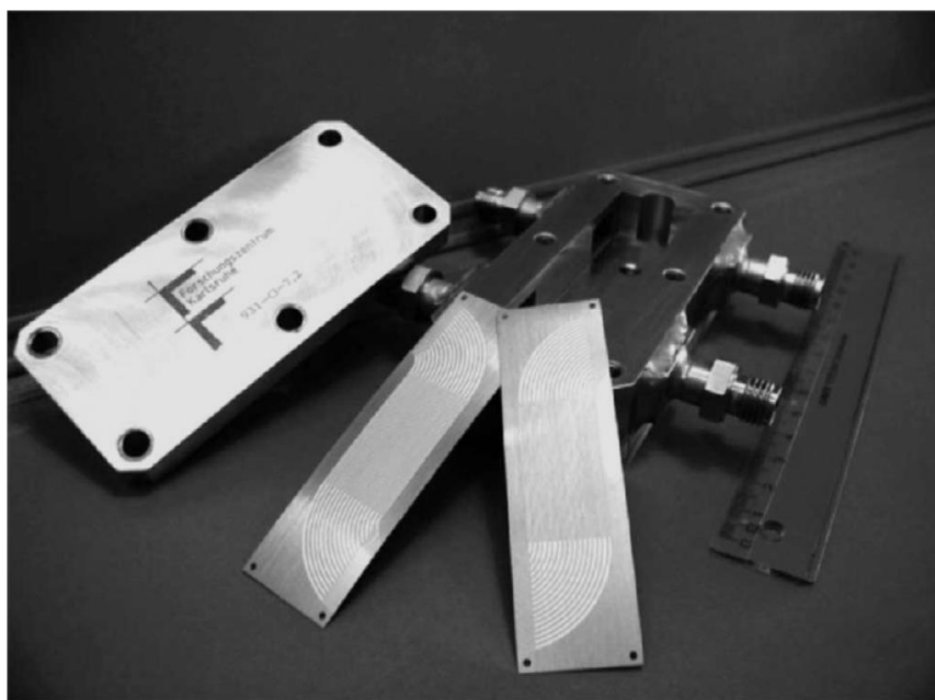
Figure 2.3 Micro-structured plates, and housing of the two-pass passage micro-structured reactor [35]
