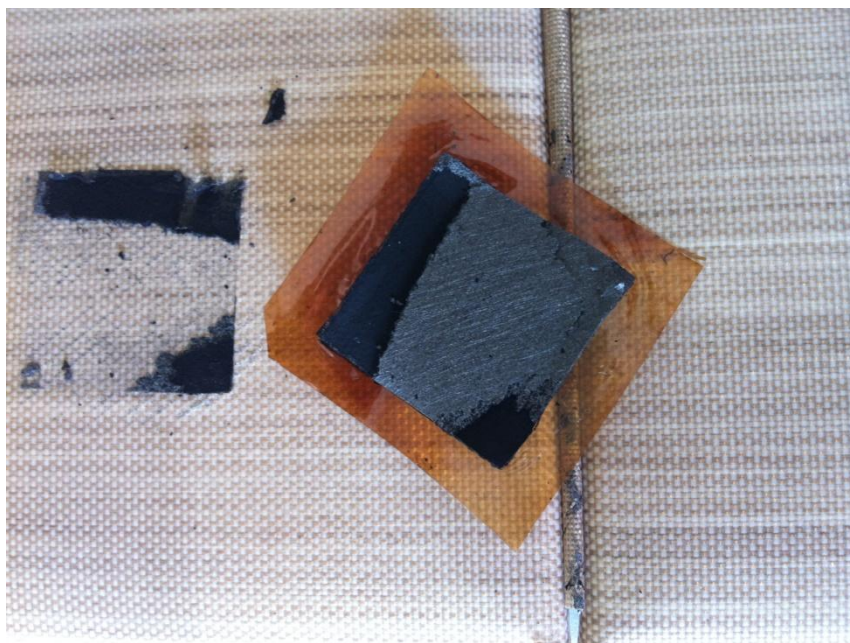
Figure 19: MEA adhesion to original silicone-covered aluminum hot-pressing plates
