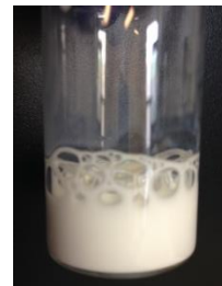
Switching-on Cycle 1 by CO 2 /5min/RT: Size=281nm, PDI=0.013, \delta =+54.7mV
