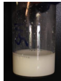
Switching-on Cycle 2 by CO 2 /5min/RT: Size=299nm, PDI=0.037, \delta =+50.2mV
