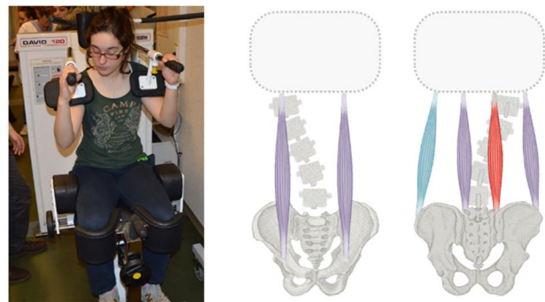
Figure 2. Muscular forces estimation: EMG calibration (left) and muscular activation (right). High activation in red, middle activation in purple and no activation in blue.
