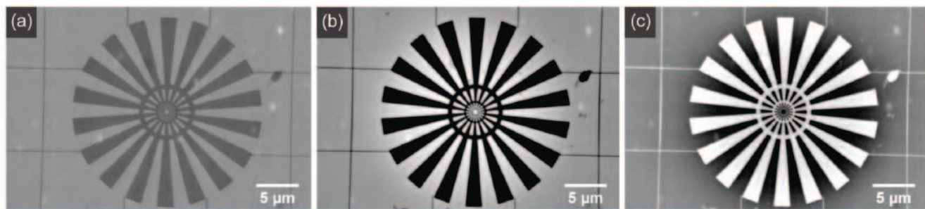
Figure 5: Full-field microscopy at 8.3 keV with absorption contrast (a) and phase contrast imaging in positive (b) and negative (c) Zernike mode [11].
