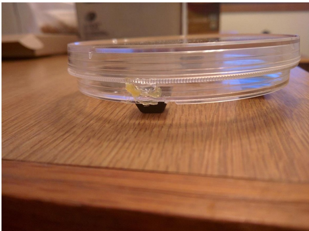
Figure 3. The 50mm opening made on the side of the cell culture dish for electrode mount.
