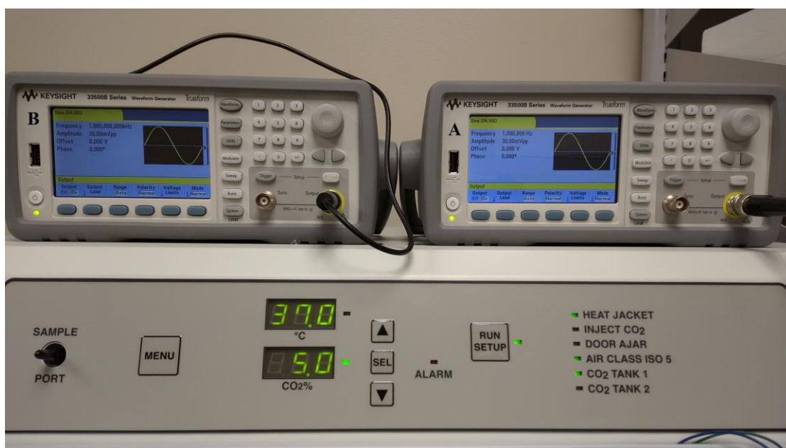
Figure 4. Waveform generator A (on the right) supplied sinusoidal 30\text{mV}_{\text{pp}} , 1Hz signal. Waveform generator B (on the left) supplied sinusoidal 30\text{mV}_{\text{pp}} , 1kHz signal to the cells. Incubator condition was set at 37^\circ\text{C} with 5% of \text{CO}_2 .
