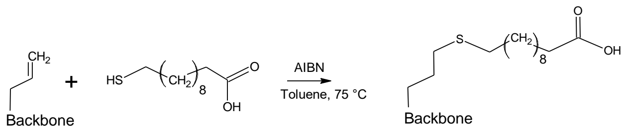
Fig. 2-7 Conversion of unsaturated mcl-PHA to carboxylated mcl-PHA with no molecular weight loss (Hany et al., 2004)
