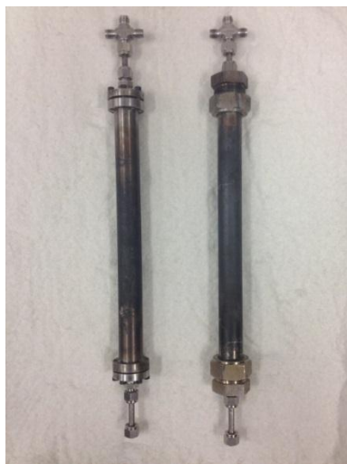
Figure 4.9: Reactor 1 with flanges on the left and the other with Swagelok fitting.
