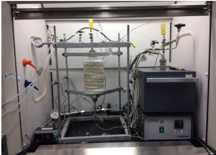
Figure 4.4: Lab-scale sulfur evaporator and sulfur-calcite reactor in RMC laboratory.
