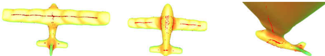
Figure 4.4: The red points are modes detected by the adaptive manifold mean shift. The model is viewed in three different angles in order to show all the detected modes.
