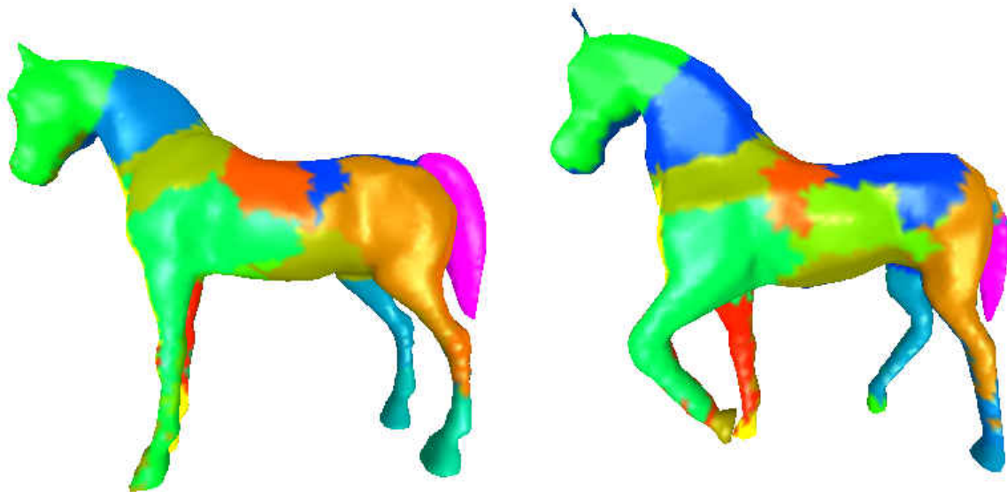
Figure 4.6: Two horse models with different poses matched with FEC decomposition and ARGs. The FEC decomposition and matching correspondence is illustrated (the matched FECs have the same color).
