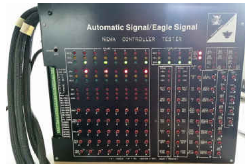
Figure 29: All-direction green lights being displayed on traffic signal test equipment. The left 4 green LEDs represent the through directions of travel at an intersection while the right 4 green LEDs represent the corresponding left-turn lanes.
