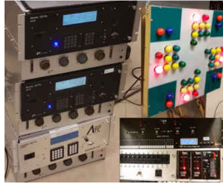
Figure 26: Traffic signal system in the municipality test lab. The left side shows a group of Model 2070 ATCs. The right top of the figure shows the traffic signal bulbs while the right bottom of the figure shows the CMU-212.
