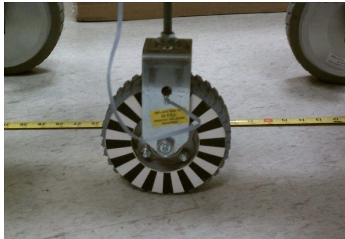
FIGURE 5.3 - THE INDEPENDENT ODOMETER FOR MEASURING DISTANCE TRAVELED
