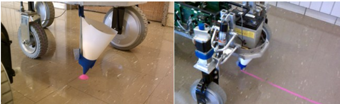
FIGURE 6.2 – THE SAND TRACER MOUNTED TO THE AXLE TRACKER (LEFT) RECORDS THE MOTION OF THE VEHICLE (RIGHT)
