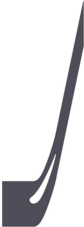
Figure 5.9: 2D Compressible Vane Geometry - Side View
