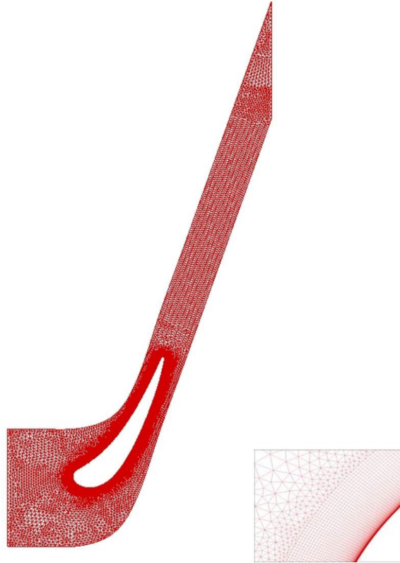
Figure 5.1: Incompressible Mesh with Detail (Kingery, Suzen, & Ames, 2010)
