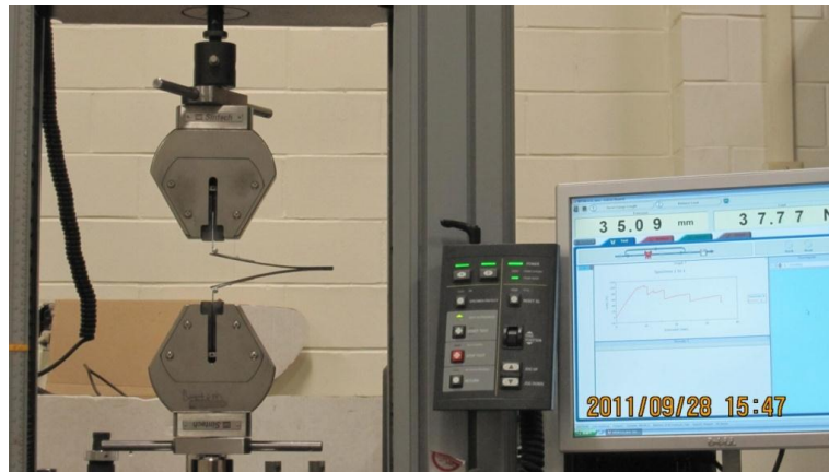
Figure 4.6. Double cantilever beam (DCB) mode I interlaminar fracture test setup.
