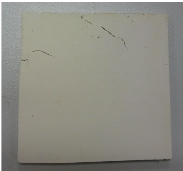
Figure 3.1. SPI/zein composite obtained from compression molding at room temperature.
