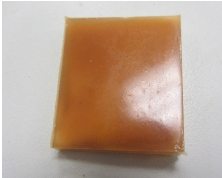
Figure 3.4. Soy/zein protein composite compressed at 130 °C.
