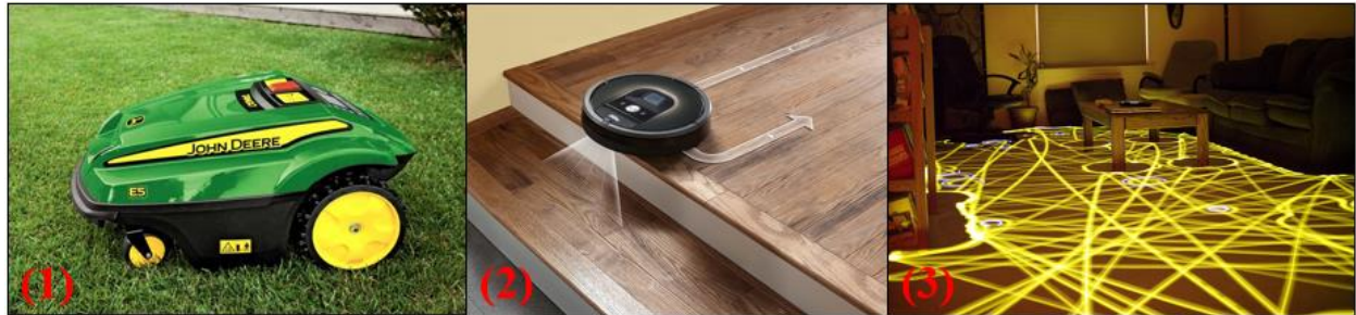
Figure 1.1: The John Deere Tango E5 can be seen in (1) and is an autonomous lawn-mower, [4]. The Roomba 960, as shown in (2), is an autonomous vacuum, [5]. Both of these robots utilize a ‘random walk’, shown in (3), which results in the inefficient completion of the task, [6], but at a large cost reduction to the cost of the robot.
