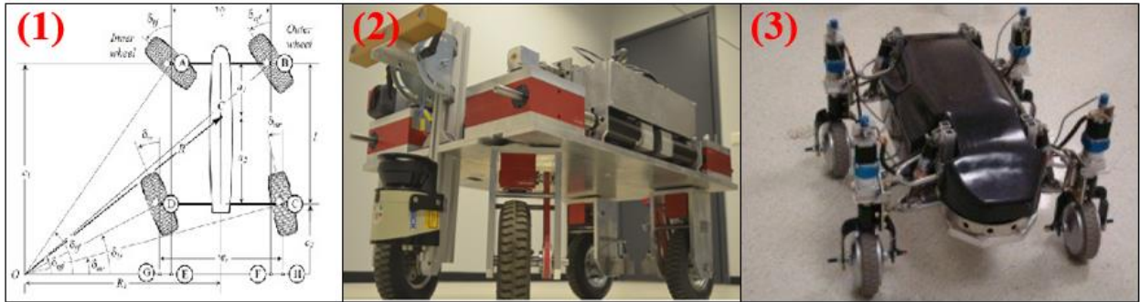
Figure 1.14: The kinematic model, [35], depicting the steering angles with respect to the ICR can be seen in (1). The iMoro, [36] mobile platform can be seen in (2). BIBOT, by NDSU Mechanical Engineering, [37], can be seen in (3).
