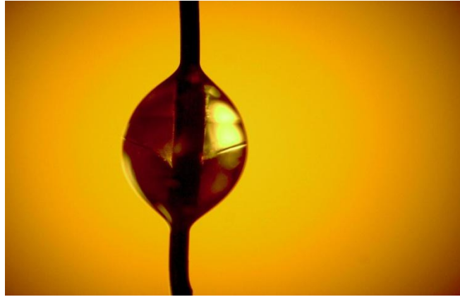
Figure 2.3. Interface between two immiscible droplets (with the assistance of Zhengping Zhou in Dr. Wu's research group at NDSU)
