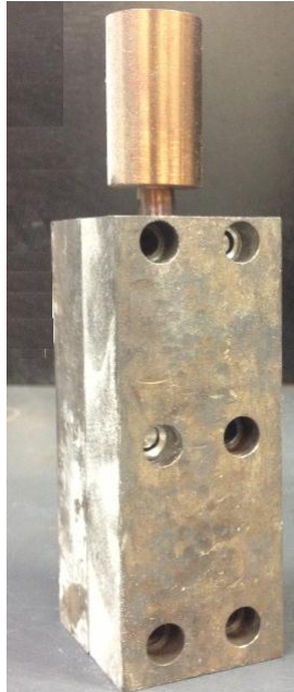
Figure 3.3. Developed die used for P/M process in this study.
