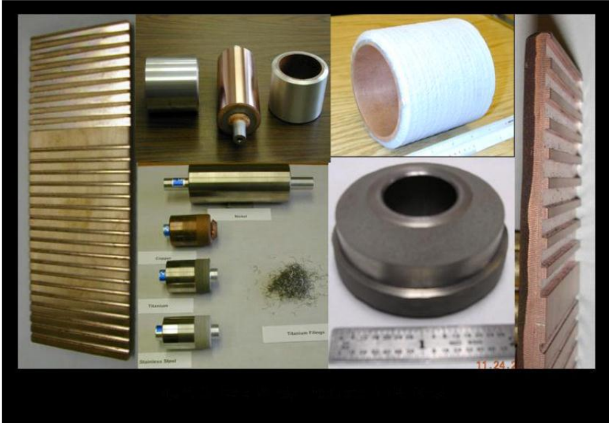
Figure 2.3. Near net shape parts fabricated using cold spray technique [10].
