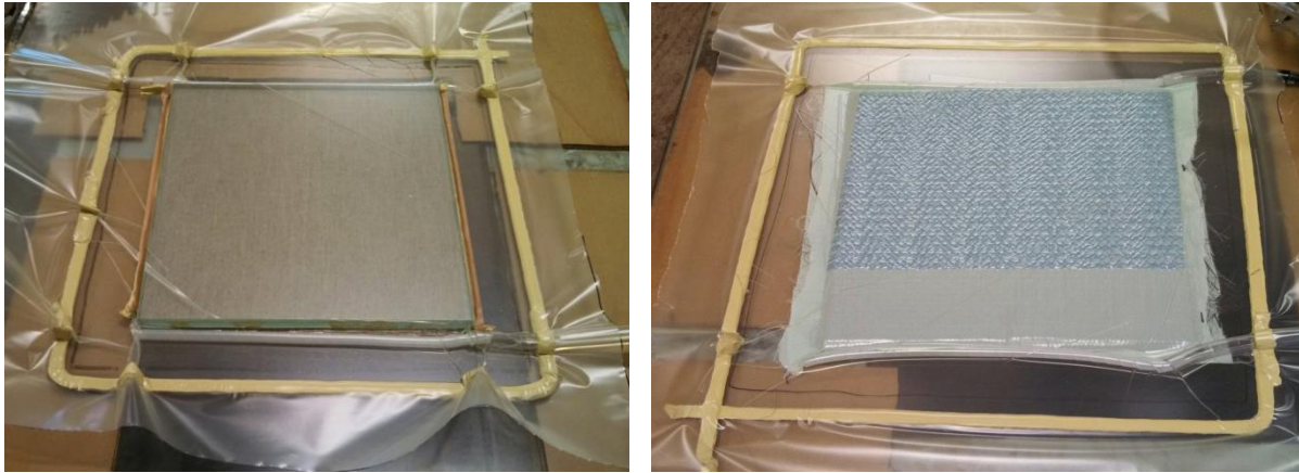
Figure 13. Typical VARTM process with caul plate (left) and without caul plate (right).
