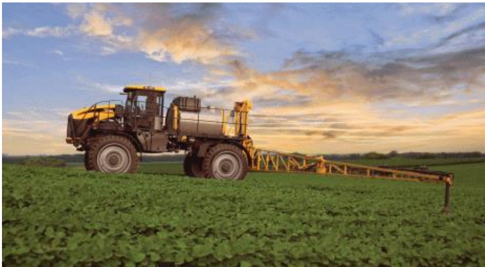
Figure 34. Agricultural sprayer boom.
