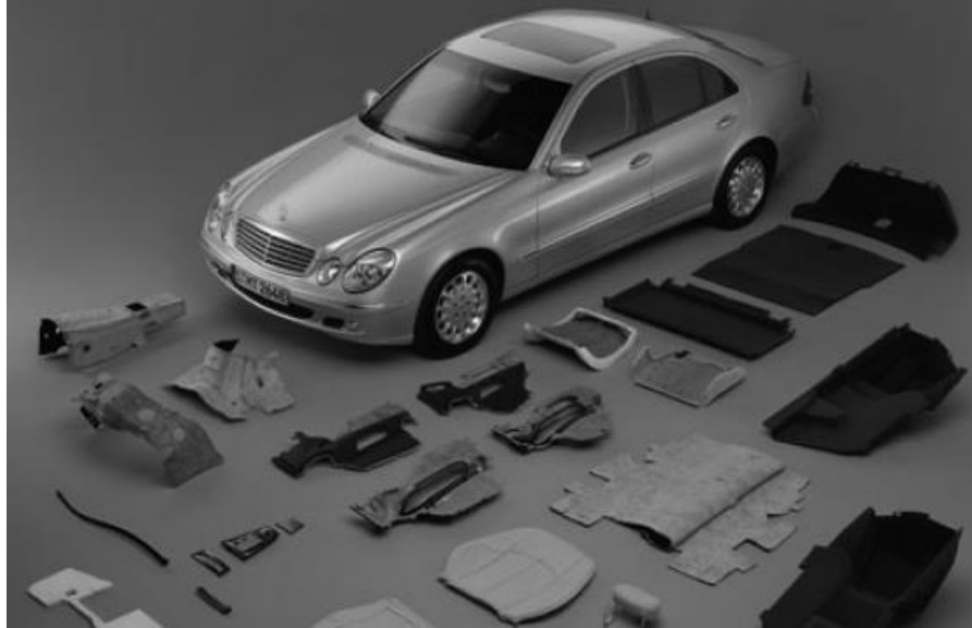
Figure 1. Flax, hemp, sisal, wood, and other natural fibers used to make various composites in the Mercedes-Benz E-Class [10].
