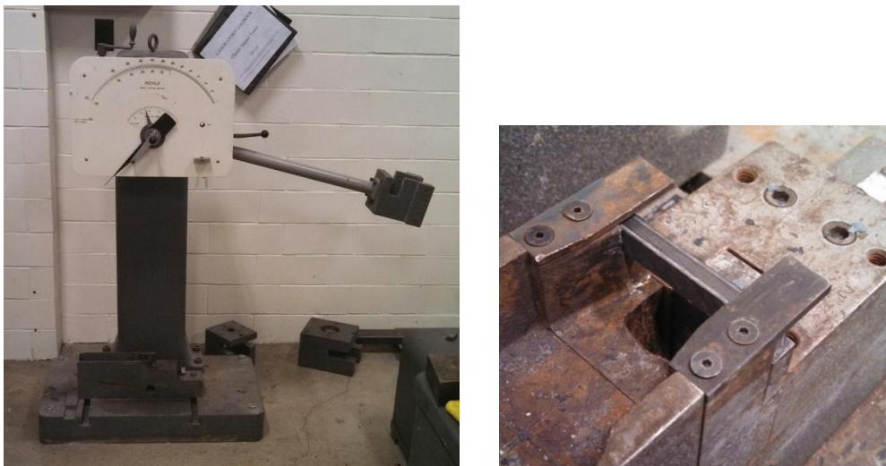
Figure 14. Reihle impact test machine (left) and an impact specimen placed in the holder prior to impact (right).
