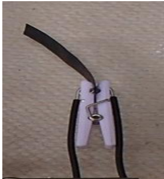
Fig. 24. Shows an IPMC specimen held by a copper electroded clamp
