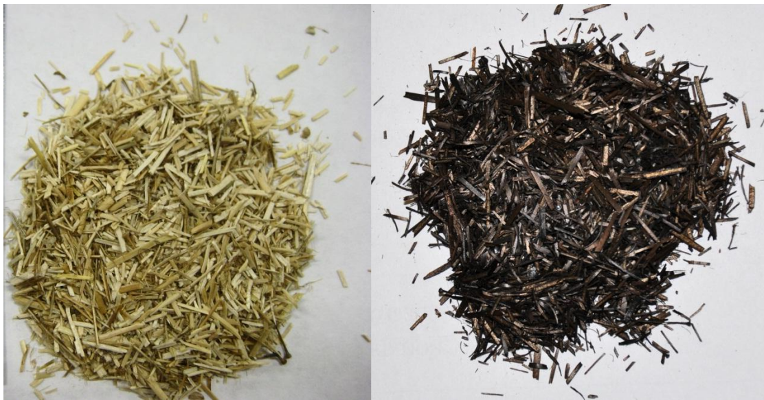
Figure 5.4: The difference between untreated flax shive (left) and torrefied flax shive (right).
