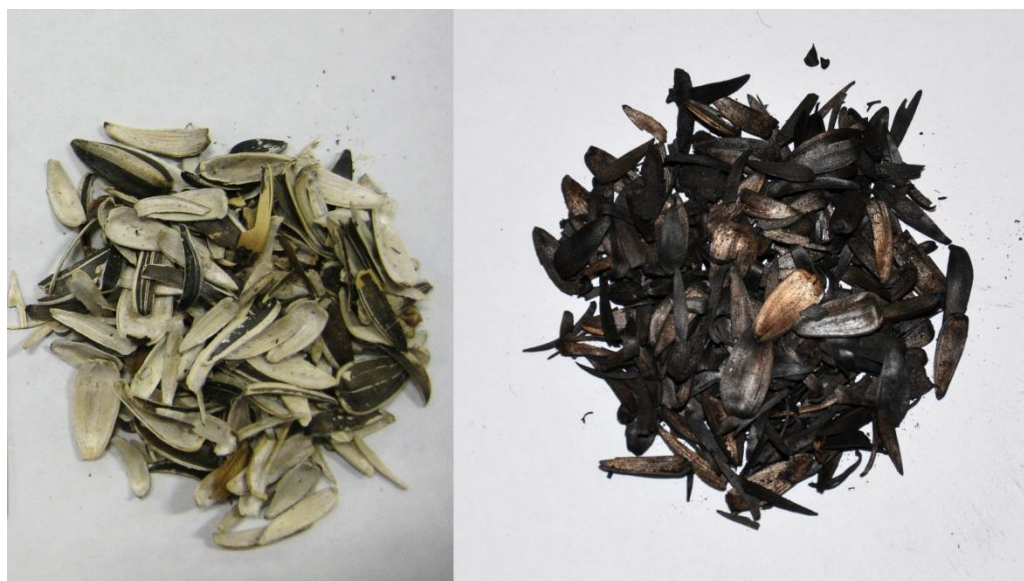
Figure 5.3: The difference between untreated sunflower hulls (left) and torrefied sunflower hulls (right).
