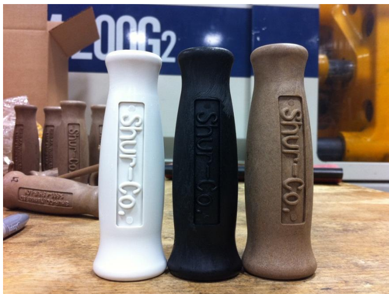
Figure 6.1: Molded final products made from neat polyamide (left) and torrefied biomass reinforced polyamide (center).
