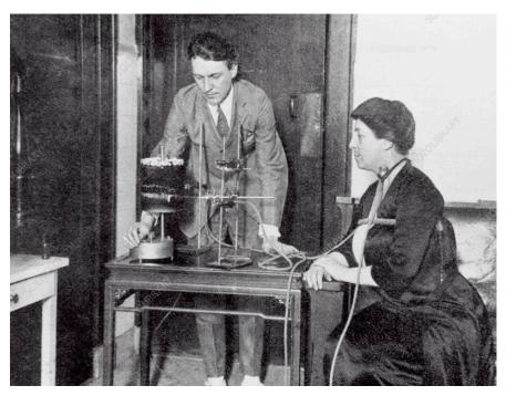
Figure 4. Kymograph in use measuring the pulse at the neck and the expansion of the lungs through the belt around the chest. The woman is a psychic medium being measured during a séance by the Society for Psychical Research, London. "Physiological measurement using a kymograph." 1920s. *SciencePhotoLibrary*.
