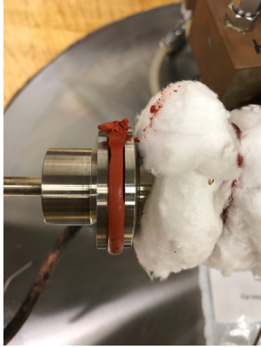
Figure 4.15: Downstream O-ring failing due to the high temperatures
