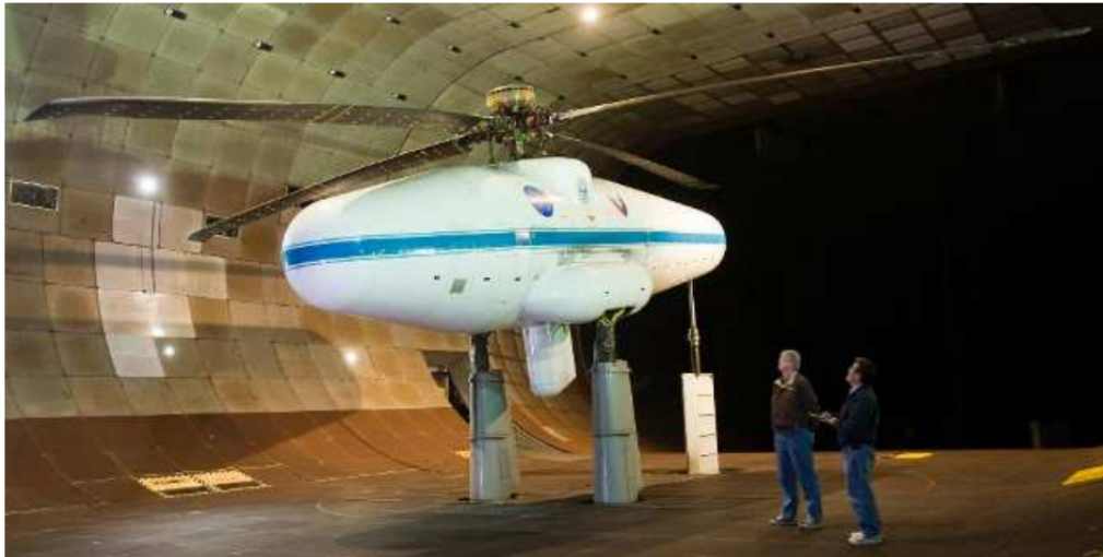
(a) The UH-60A rotor system installed in the National Full-scale Aerodynamics Complex (NFAC) 80 ft x 40 ft wind tunnel.
